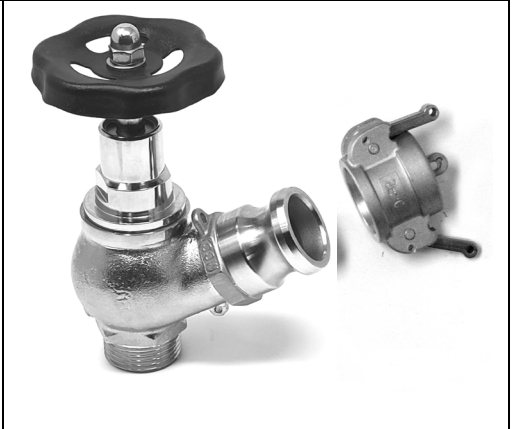
#91.778 Valve 1 inch showing with Stainless Steel Camlock Coupling & cap Steel powder coated turning wheel Thread: 1" BSP. Valve chrome plated brass
