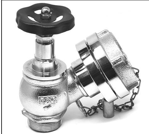
#91.778 Valve + 1 1/2" with N=66 Storz Coupling and Dust cap Steel powder coated turning wheel Thread: 1 1/2" BSP. Valve chrome over brass
