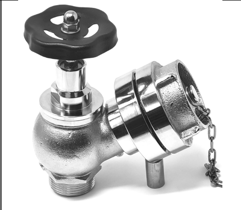
#91.778 Valve 1/4" showing with Storz coupling and dust cap N=52 Steel powder coated turning wheel Thread: 1 1/4" BSP. Valve chrome plated brass
